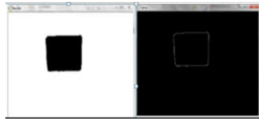
Fig. 4: Gaussian filter and Canny algorithm
