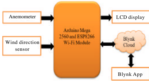
Fig. 5: Block diagram of crosswind detection monitoring system
