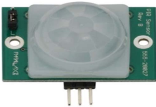
Fig. 5: PIR motion sensor
