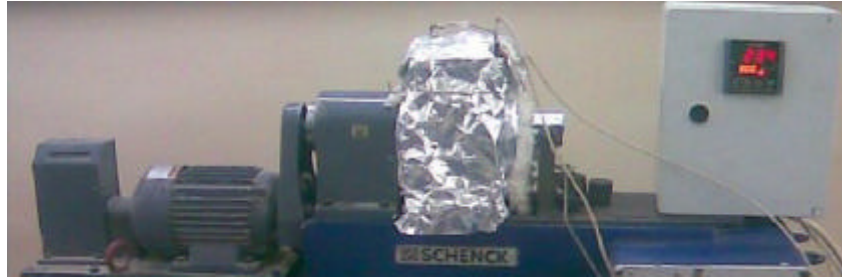
Fig. 3: Furnace attached to fatigue machine with control board
