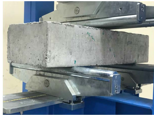
Fig. 5: Ribbed slab experimental set up
