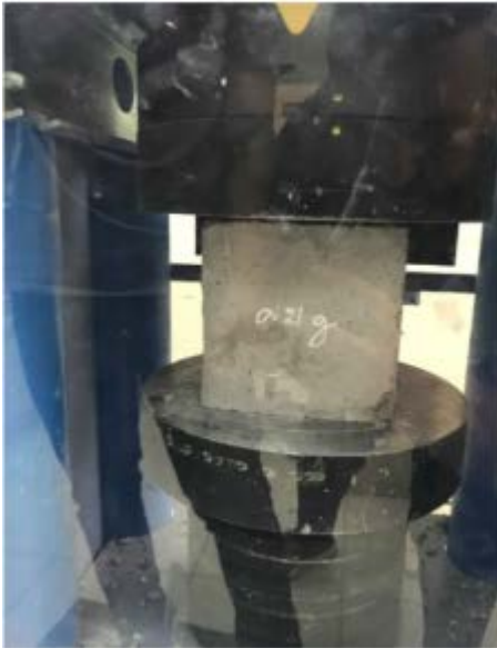
Fig. 3: Concrete cube is tested for compressive strength
