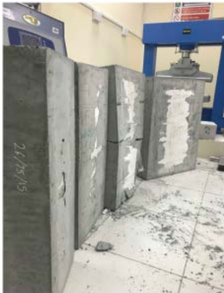
Fig. 12: Ribbed slabs of variable width after failure
