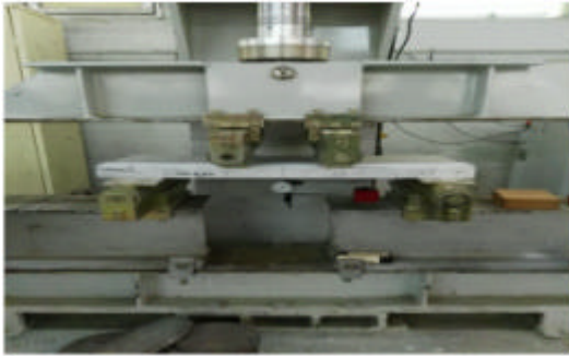
Fig. 6: Test set-up of ferro geopolymer slab
