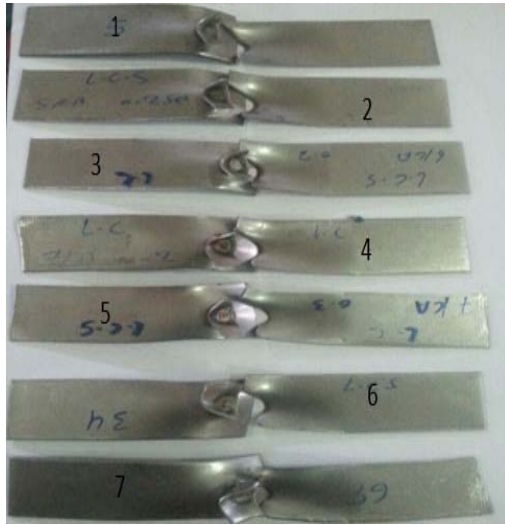
Fig. 13: The failure mode of shear test
