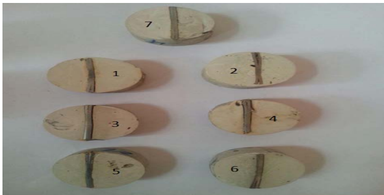
Fig. 2: Sample for microstructure and hardness
