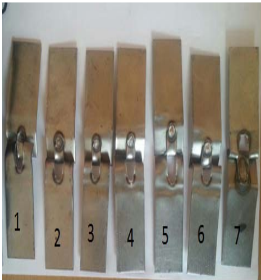
Fig. 14: The failure mode of peel test
