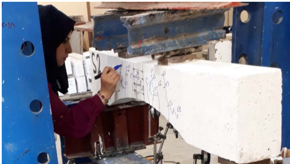
Fig. 5: Recording the development of cracks
