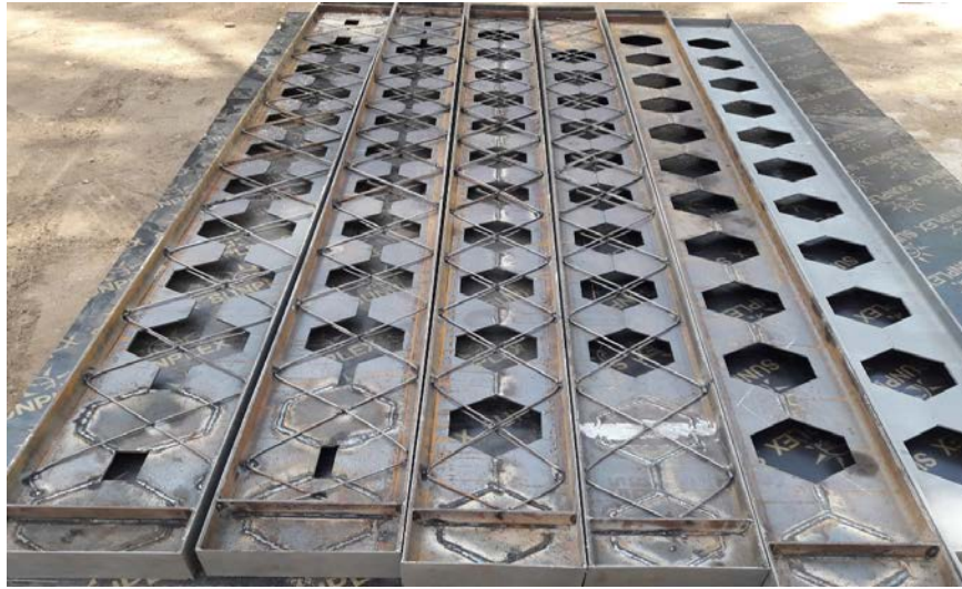
Fig. 2: Fabricated castellated steel beams
