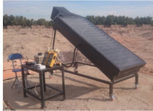
Fig. 2: Photograph of the experimental setup for corrugated solar air collector
