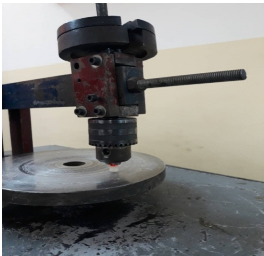
Fig. 2: Pin on disc machine used for wear test
