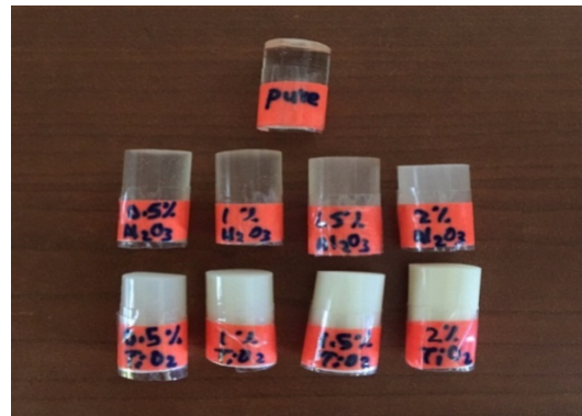
Fig. 3: Pins used in wear tests with different particle concentrations of \text{Al}_2\text{O}_3 and \text{TiO}_2
