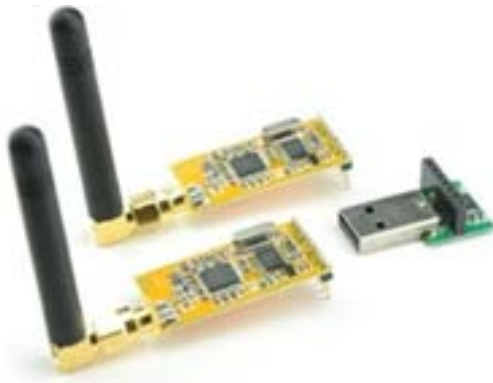
Fig. 5: APC220 module communication (Yamato et al. , 2008)
