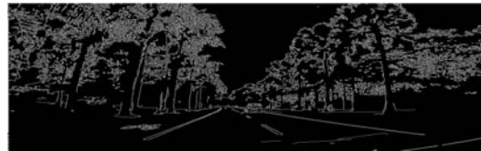
Fig. 11: Result of Canny edge detection on image
