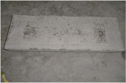
Fig. 2 a, b): Surface preparation for the strengthened specimens
