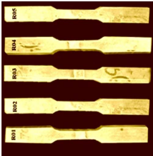
Fig. 4: Specimen for ultimate tensile strength
