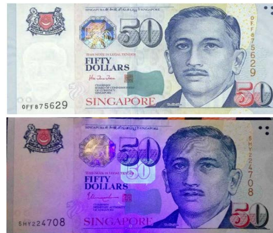
Fig. 3: An example of money is 50 Singapore dollars before it is irradiated by UV rays and after being irradiated by UV rays
