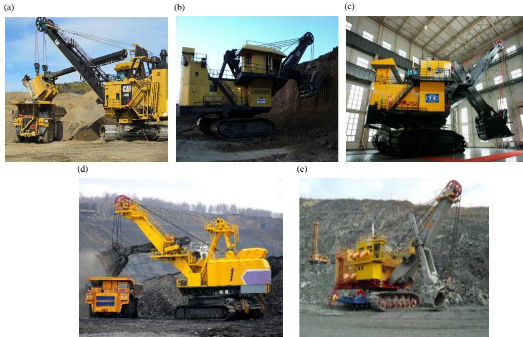
Fig. 4: Rope excavators with front shovel: a) Caterpillar; b) P&H; c) TYHI; d) IZ-KARTEX and e) Uralmashplant
