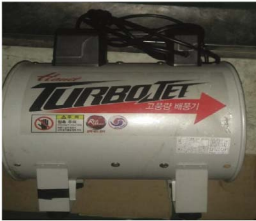
Fig. 7: Ventilator used for ammonia gas discharge
