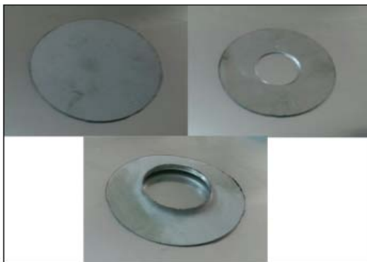
Fig. 3: Manufacture steps of fins
