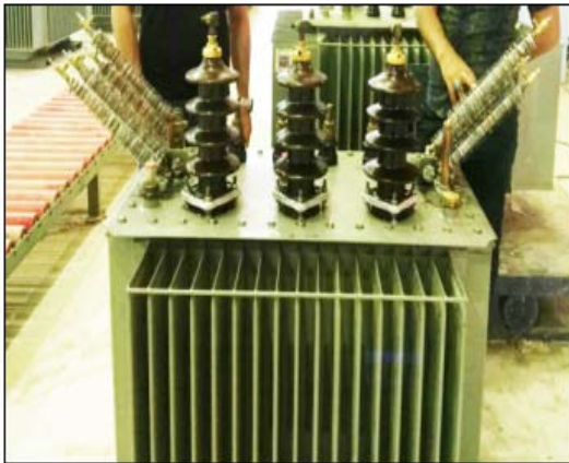
Fig. 7: The last shape for transformer with thermosyphon
