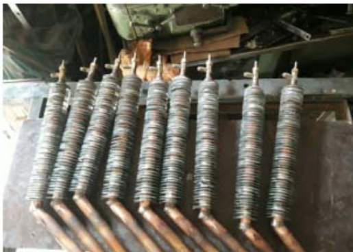
Fig. 2: Thermosyphon with 40 fins at 45° angle of inclination
