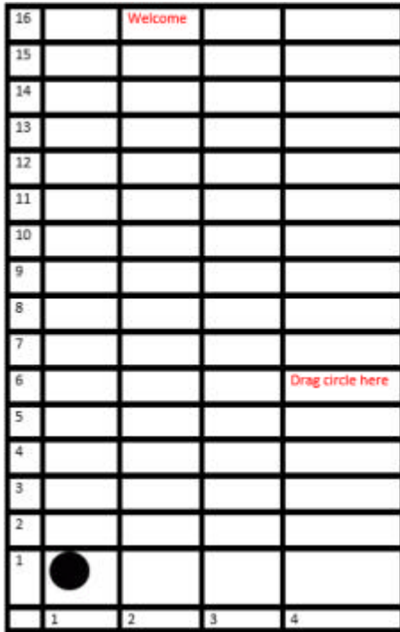
Fig. 4: Proposed drag and drop CAPTCHA on a 16*4 pixels display
