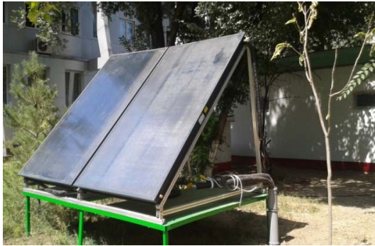
Fig. 2: Full-scale model of a solar collector
