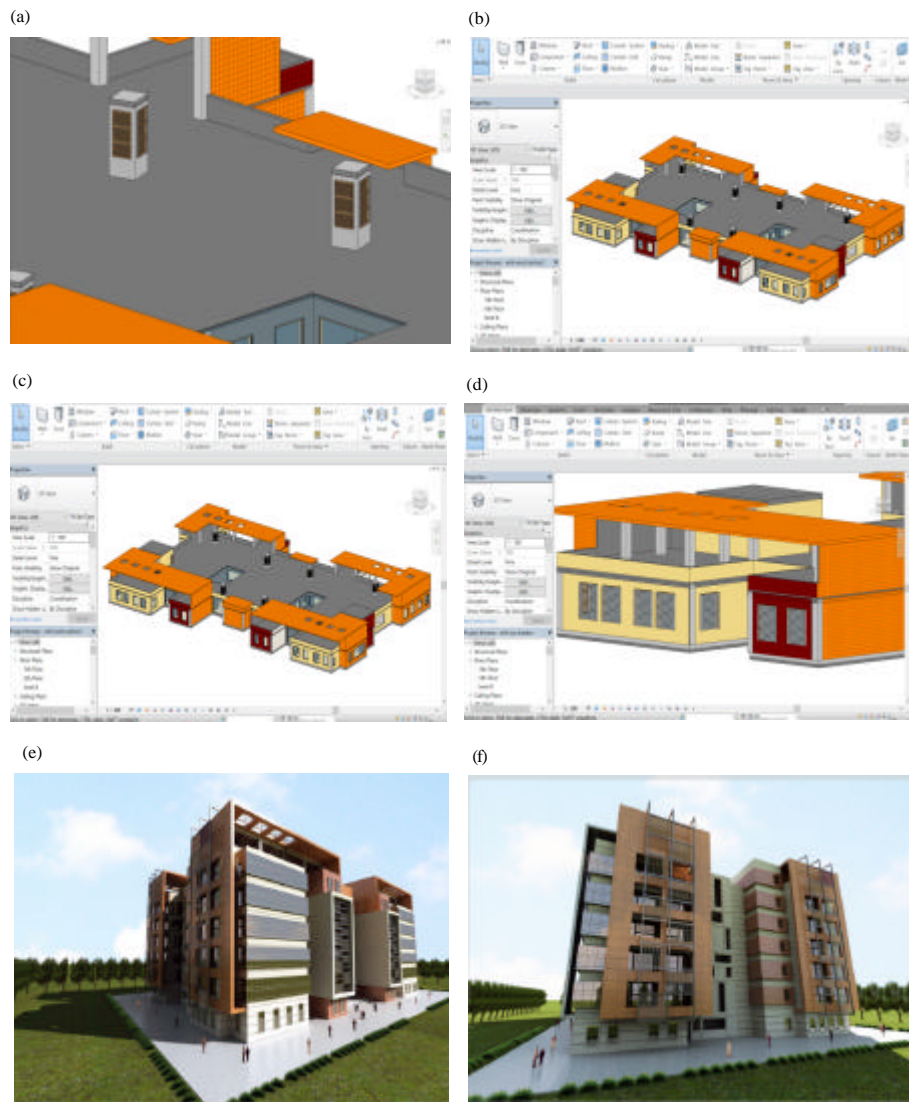
Fig. 9: a-f) The addition of new design elements (solar breakers, spacers and roofing)
