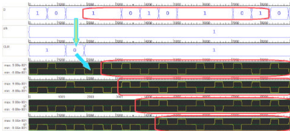
Fig. 20: Simulation results of SIPO shift register using QCA clocked D-FF with clear
