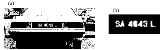
Fig. 3: Detection process (detection): a) Binary image and b) (Output) plate location
