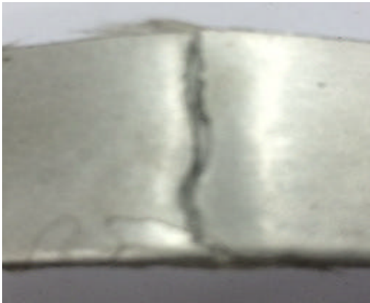
Fig. 6: Fracture surface under bending load for both tested FMLs
