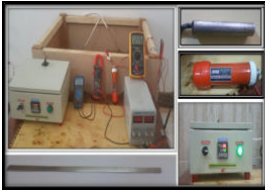
Fig. 2: Model of Impressed Current Cathodic Protection (ICCPs)
