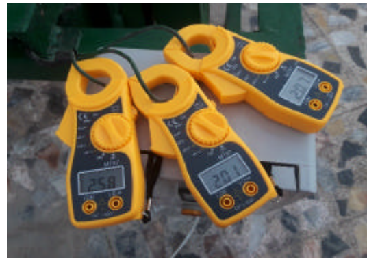
Fig. 16: The clamp-meters used to measure the electric current of the manufactured testing machine
