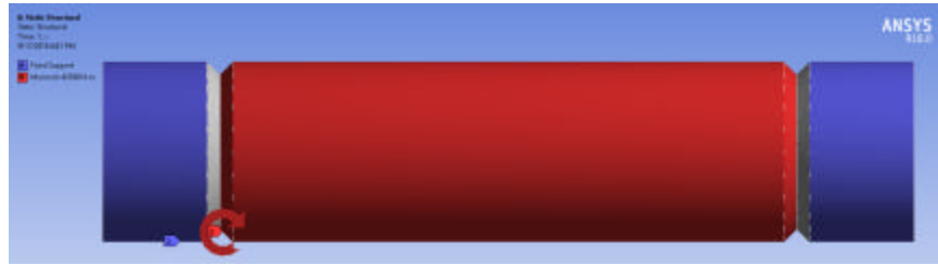
Fig. 26. Fracture torque of ( 2\bullet = 90^\circ , d = 5 , \bullet = 0 ) compute by ANSYS to equal (40.12 kNm)
