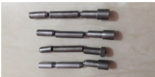
Fig. 21: Samples of shear pins fractured by the testing machine
