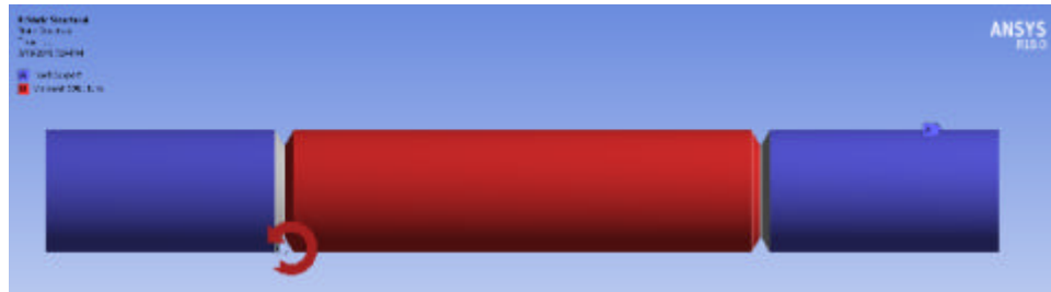
Fig. 18: The numerical torque fracture of the shear pin that used in manufactured testing machine (2• = 60°, d = 2 mm)
