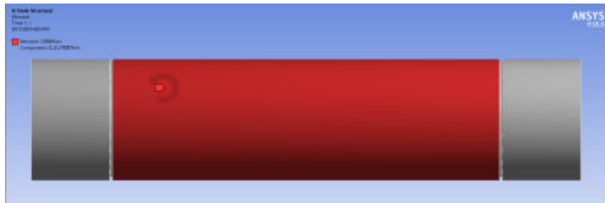
Fig. 22: Fracture torque of ( 2\bullet = 30^\circ , d = 2 , \bullet = 0.5 ) compute by ANSYS to equal (27 kNm)
