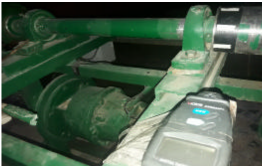
Fig. 17: Digital tachometer that used to measure the rotating speed through the testing process
