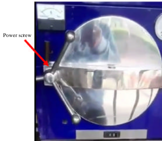
Fig. 2: Compression by power screw
