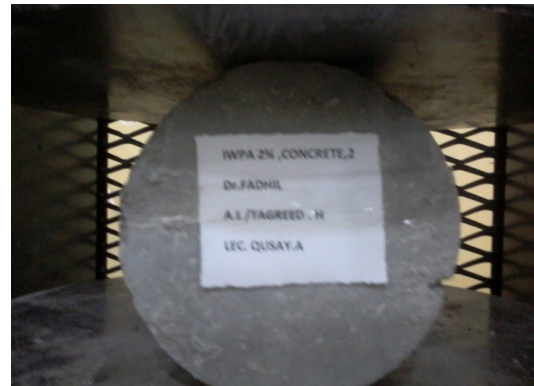
Fig. 3: Cylindrical IWPA concrete specimen under tensile test
