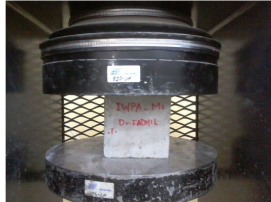
Fig. 2: Cubic concrete specimen under compressive strength test
