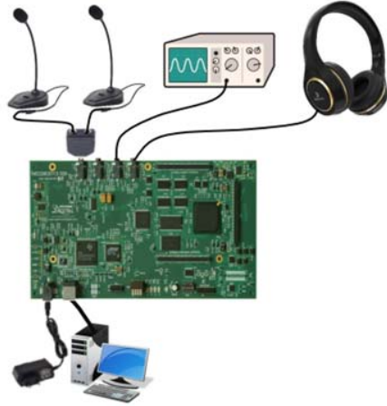
Fig. 4: Hardware setup for system separation
