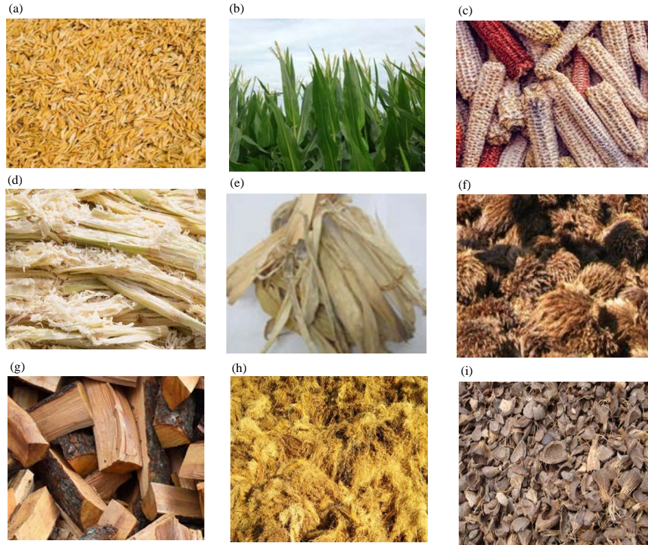
Fig. 1(a-i): Different categories of biomass residues for power generation (a) Rice husk, (b) Corn stalk, (c) Corn cob, (d) Sugarcane bagasse, (e) Corn straw, (f) Palm empty fruit bunch, (g) Forest firewood, (h) Palm pressed fiber and (i) Palm shell
