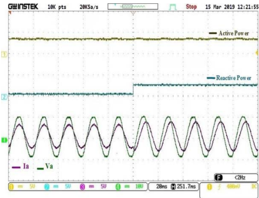
Fig. 36: Laboratory results of the changing step for the reactive power where the active power has fixed value [Scale: V: 150 V/div, I: 5 A/div, P: 1000 W/div, t: 20 msec/div]
