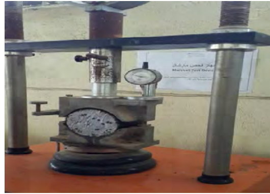
Fig. 4: Marshall stability test
