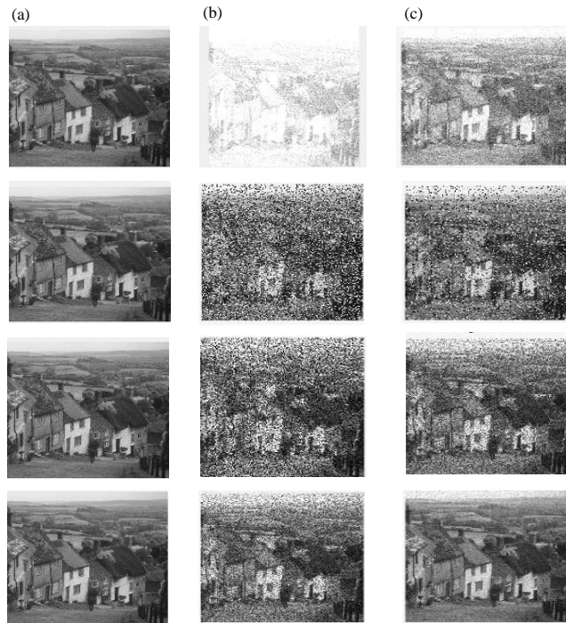
Fig. 6 (a-c): Denoising of Goldhill image corrupted with 70% noise density (a) Original image (b) Noisy images and (c) Corresponding denoised image by the proposed system
