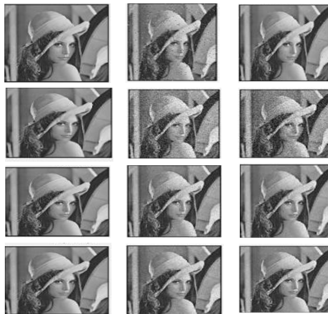
Fig. 3 (a-c): Denoising of lena image corrupted with 10% noise density (a) Original image (b) Noisy images and (c) Corresponding denoised image by the proposed system
