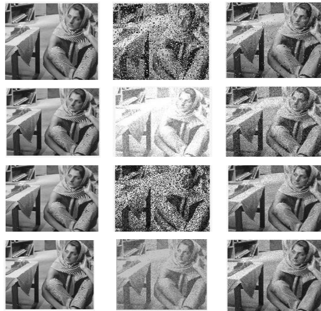
Fig. 5 (a-c): Denoising of Barbara image corrupted with 50% noise density (a) Original image (b) Noisy images and (c) Corresponding denoised image by the proposed system
