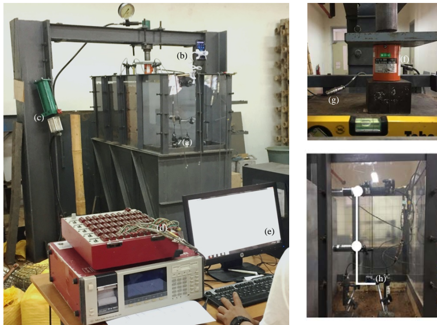
Fig. 2(a-h): Testing apparatus of physical model, (a) Testing tank, (b) Loading frame, (c) Hydraulic pump, (d) Data Logger, (e) PC desktop (f) Load cell 100 kN (g) Loading plate 20 mm and (h) LVDT
