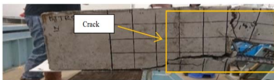
Fig. 1: The crack at the support area
