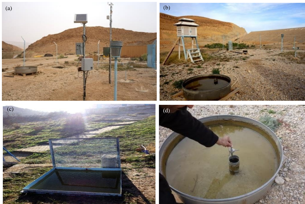
Fig. 2(a-d): Existing evaporation pans in the studied dams, (a) Weather station of Fom El-Gherza dam, (b) Weather station of Fontaine des Gazelles dam, (c) Colorado pan-Foum El-Gueiss dam and (d) Class-A-pan-Fontaine des Gazelles dam
