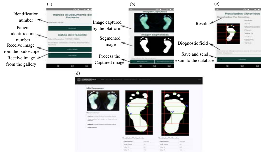
Fig. 6(a-d): Graphic interface of the mobile application; a) Receiving data; b) Exam display screen; c) Display screen of the results and d) Exam and results page in the web page
