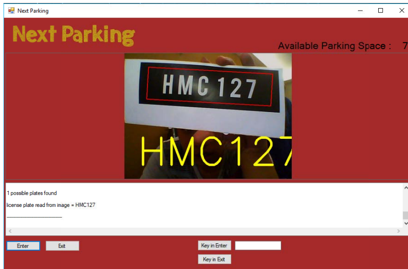
Fig. 3: The proposed next parking system with car plate number capture at entrance of the parking
