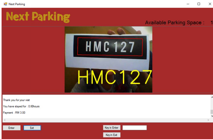
Fig. 4: Next parking system with capture at exit of the parking with the total parking charge
