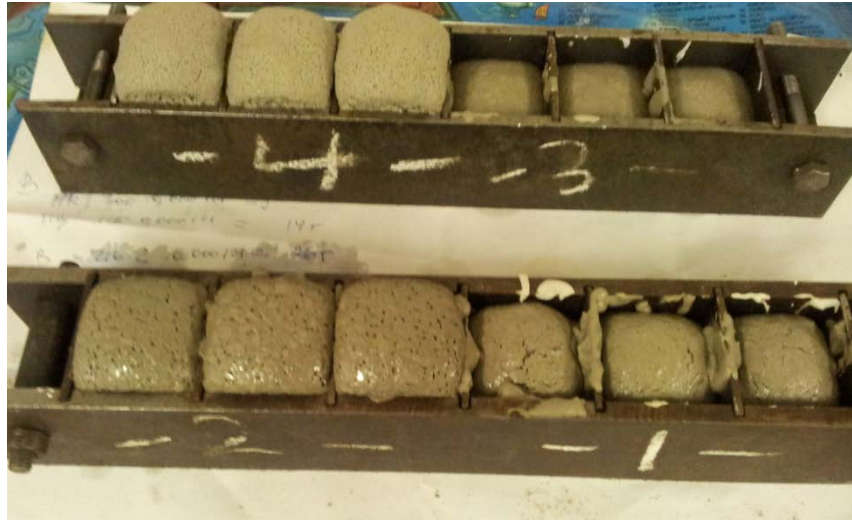
Fig. 7: Extrusion of aerated concrete samples in molds
