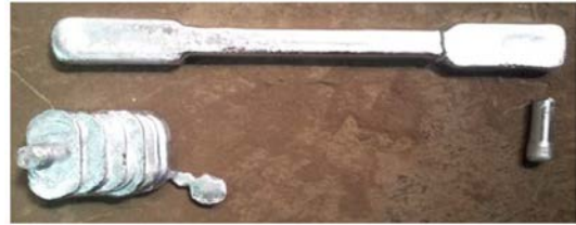
Fig. 4: Aluminium casting results that fail after removal from the mold
