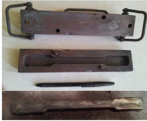
Fig. 2: A pair of molds (top) and specimen (bottom)
