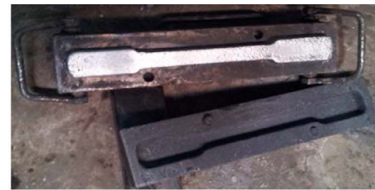
Fig. 6: Aluminium scrap castings are easily removed after the bottom mold is sprayed with graphite powder
