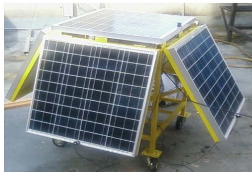
Fig. 2: System modules into four direction slope angle (30°)
