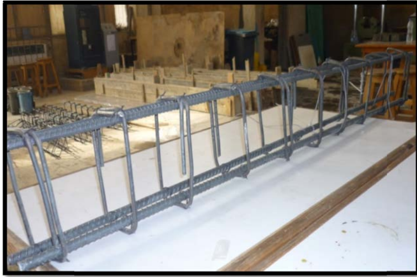
Fig. 3: Reinforcement details of beam
