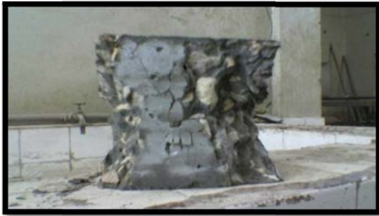
Fig. 4: Standard cube failure shape
