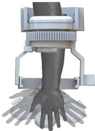
Fig. 12: Adduction and abduction movement of the exoskeleton
