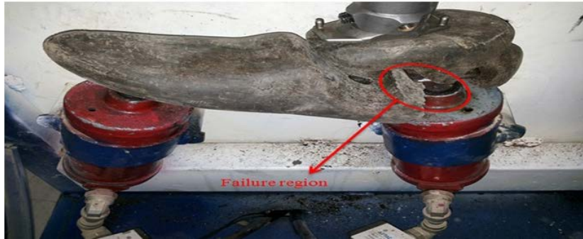
Fig. 5: Failure region in non-articulated foot (HDPE+LLDPE)
