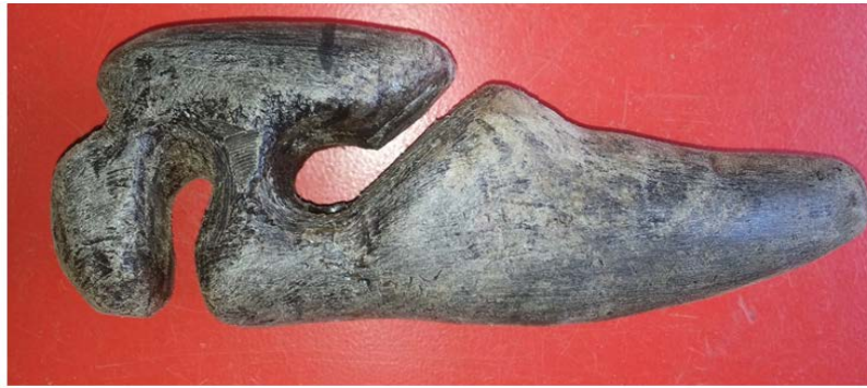
Fig. 1: The injection foot blended of (DPW+HDPE)
