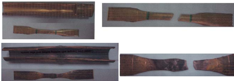
Fig. 4: The tensile testing specimens for different diameters
