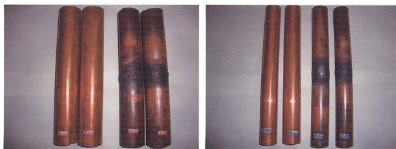
Fig. 2: Copper pipes before and after welding processes
