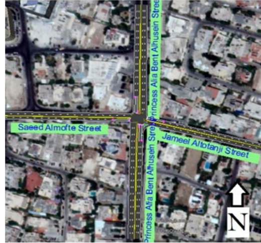
Fig. 8: The base model development of Alaqsa Intersection using synchro
