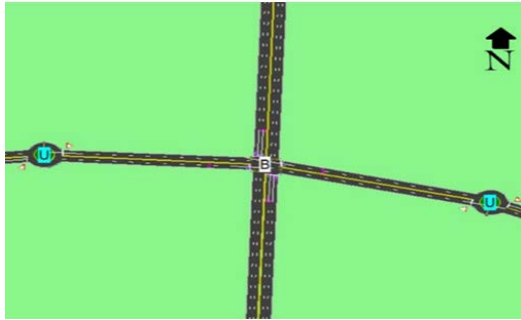
Fig. 13: The LOS at Ebad Alrahman Intersection when use the bow-tie intersection
