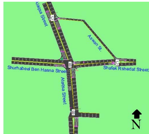
Fig. 12: The LOS at Alaqsa Intersection when use Jug-handle Intersection
