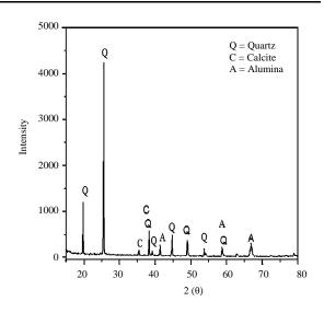
Fig. 1: Diffractometry analyses of dune sand
