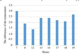
Fig. 9: The difference between the interior temperature and the external temperature of the prototype P1
