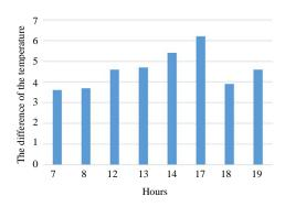
Fig. 13: The temperature difference between the inside and the outside of the prototype P3
