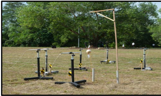
Fig. 6: Field blast test set up
