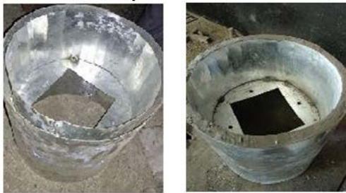
Fig. 7: Manufacturing of skirt for stove
